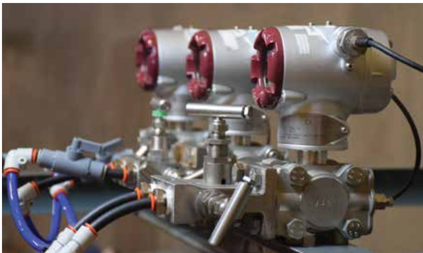
▲ Figure 3. A bank of smart differential pressure transmitters. Courtesy of Azbil North America
